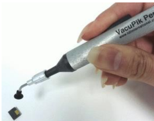
Figure 8: Example of vacuum suction pen
